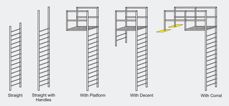
NOTE: The latest OSHA codes require all fixed ladders above 24' in height must be equipped with lifelines. For a **complete** fixed ladder solution, check out our Fixed Ladder Lifelines.
