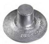
A spigot flange which fits inside the pipe and is not secured by a set screw. Type 59 can only be used with a pipe wall thickness of 1/8" and in light, self supporting structures.
