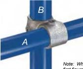
Designed to give a 90° crossover joint. Frequently used on safety railing where, to reduce cost by minimizing the pipe cuts, a continuous horizontal rail is used. Pipe cannot be joined within this fitting. It may also be used to give intermediate levels on racks etc. when horizontal ties between uprights are not required.
