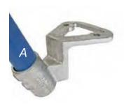
A component designed to retrofit roof parapets that are an unsafe height. Rail anchor is angled 25 degrees from the vertical so that the building's visage is unaffected by the implemented railing. Two holes are located in the top mounting bracket for mounting directly into the parapet. The two set screws in the vertical socket give greater side-load stability to the angled upright. Engineered weep hole allows water to drain.
