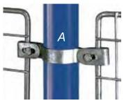
For attaching wire-mesh in-fill. For economy it is possible to use Type 82 clips without the safety attachment, to secure various types of in-fill panels (ply-board, PERSPEX, etc.) up to a thickness of 25/64". All clips are supplied with hexagonal head fixing bolts, M6x35mm long, and nut. The primary clip has a slot measuring 8mm x 15mm.
