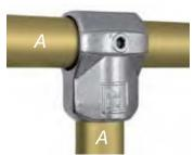
Designed to give a 90° butt joint between two pipes. Frequently used for the joint between end uprights and the middle rail where the railing site is straight and level. Also used for base ties on racking. This fitting cannot be used where the pipe through sleeve 'A' is required to be joined within the fitting.
