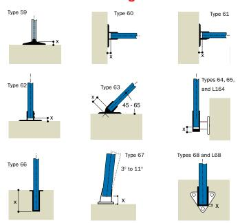
Table 13 gives details of the ground fixing dimension 'x', to be subtracted from the height 'H' to give the length of the upright 'h'.
