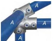
The Type 350 fitting has been designed for small structural building applications and provides for significant load rating. When used with the Type 351 ridge fitting a truss arrangement for additional support can be achieved. Double set screws are provided on the truss outlet to provide additional pull out resistance to hold structures firmly together.
