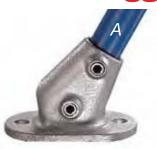
Similar to Type 62, but used to set up the upright at an angle between 45° to 60°. This fitting should only be subjected to light loads which cannot be positioned at 90° to the applied load. For greater loads or other pipe sizes, a Type 62 flange is used and the upright bent to the required angle (refer to table on page 43).
