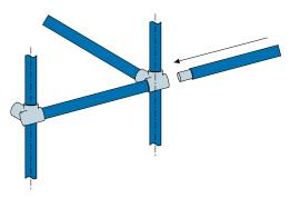
Spigots can be either pipes or rods, riveted into position, or the Type 18 fitting. When using the latter, a gap of 3/4" must be allowed for the set screw fixing.
