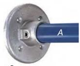
Heavy duty flange with wide base for spreading loads over a large surface area. Hole provided for countersunk flat head screw fixings only, for use on structures where the fixing required is positional only. Frequently used as a wall fixing bracket (refer to table on page 43).
