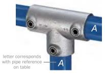
Most commonly used as the 90° joint between the top rail and an intermediate upright on safety railing. As there are two socket screws in the sleeve, this fitting can be used where a join is required in the horizontal pipe. The Type 10 fitting can be used as an alternative when a join in the pipe is not required.
