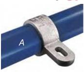
Designed for the securing of various types of panels and flooring to pipe structures (ie. plywood, plastic sheeting, wood planking, etc.). This fitting has a single offset flange to allow for the attachment of panels to pipe. See Type P50.
