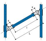
Table 10 gives details of dimension 'x' to be subtracted to give the pipe length required for use with two Type F50 or LF50 fittings in the formula I - L-2x.
