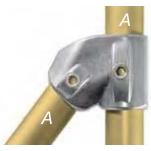
This adjustable fitting is most frequently used for struts and braces. It can be used at any selected angle between 30° and 60°. Suitable for connecting an angled staircase rail to a vertical upright.
