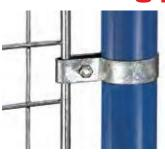
For attaching wire mesh in-fill. For economy it is possible to use Type 81 clips without the safety attachment to secure various types of in-fill panels (ply-board, PERSPEX, etc. ) up to a thickness of 25/64". All clips are supplied with hexagonal head fixing bolts, M6x35mm long and nut. The primary clip has a slot measuring 0.31 x 0.59 inches.
