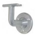
Designed to provide attachment for a smooth handrail which complies with the Americans with Disabilities Act of 1990. Three fixing holes are drilled and countersunk to suit 1/4 in. diameter flat head wood screws. Designed for use with size 7 pipe.
