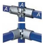
This fitting performs the same function as either Type 21 or Type 26, but because of its unique hinge pin system, it can be added to an existing tubular assembly. Type A21/A26 fittings are supplied and priced as a kit including two casting and two taper pins, which can be assembled in either configuration.
