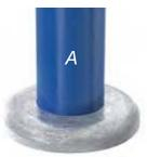
This fitting slips over uprights to finish below ground post installations. The fitting is secured to the upright pipe with a single recessed set screw.
