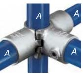
The unique hinge and pin system of this fitting enables existing structures to be easily extended without the need for dismantling. This fitting has been designed to tie an upright with horizontal pipes in three directions, all at 90° to the upright. The upright passes through the fitting.
