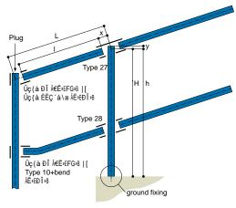
Table 2 gives details of dimensions required for calculating the rail lengths, where angles are between  $0^{\circ}$  and  $45^{\circ}$ .
