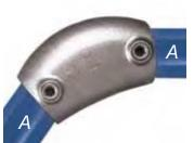
The Type 55 is an ideal fitting to use as an alternative to bending, or when a junction between a sloping pipe and an end post is required, ie. guardrail and staircases (Refer to page 41 for more information).
