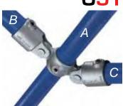
Complete combination fitting. Type C51 is made by combining two Type F50 fittings and one Type M51. For dimensions refer to Type F50 and Type M51. See 'Swivel Fittings' on page 12 for more information.
