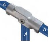
Used for safety railing on slopes between 0° and 45°, between the top rail and an intermediate upright which is required to remain vertical. Components are held in stock as blanks and then machined to individual requirements.
