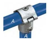
Designed to allow additions or extensions to existing structures without the need for dismantling. Pipe must not be joined within the fitting. Fitting has strength and function comparable to Type 10 components.
