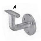
A wall mounted version of the 518-7. The handrail tube sits on the 'saddle' and is secured using either No. 12 selfdrilling screws or multi-grip pop rivets. This bracket provides holes for countersunk head fixing screws only. Three fixing holes are drilled and countersunk to suit 1/4 in. diameter flat head wood screws.
