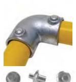
Aluminum drive rivets deter tampering with set screws as well as create a finished, aesthetic look. Drive rivets are easy to install, requiring no special tools. The drive rivet is set by striking the pin with a hammer, driving the pin flush with the rivet head and expanding the back side of the rivet. One size fits components 5-9. Rivets for components 2-4 available upon request.
