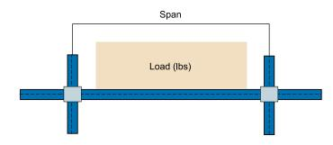
Table 17 gives an indication only of the safe load, uniformly distributed, in pounds, that may be carried per shelf consisting of front and back pipes when used as continuous beams.
