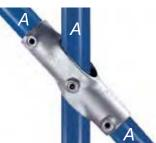
Designed as an alternative to the Type 28 fitting, this adjustable fitting can be used for railing on staircases between the mid-rail and an intermediate upright which is required to remain vertical. It may be used at any selected angle between 30° and 45°.
