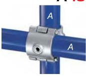
The unique hinge and pin system of this fitting enables existing structures to be easily extended without the need for dismantling. This fitting is designed to give a 90° offset crossover joint. Pipe should not be joined within the fitting. Type A45 function is comparable to Type 45 fitting.
