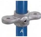
This fitting can be used for attaching flat panels to tubular structures. Specially designed for retail shelving applications, the MH51 can be used as part of a CH51 combination fitting.
