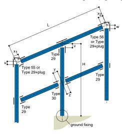
Table 6 gives details of dimensions required for calculating the rail lengths, where angles are between 30° and 45°.
