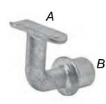
An intermediate upright handrail support. This bracket is designed to be mounted on a Type 10-848 or a Type A10 fitting; the rail sits on the saddle and is secured by either Ø4.8mm x 15mm long aluminum 'multi-grip' pop rivets or No. 10 x  $m{B}$  20mm countersunk self-tapping screws.
