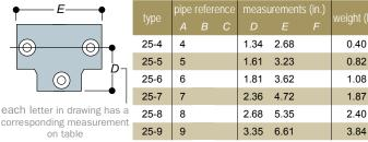
first number preceding the dash identifies the component type — single digit following the dash defines pipe size. (Two digits after the dash indicate that the fitting is designed to receive two sizes of pipe, and likewise with three digits.) See below for pipe reference digits related to actual pipe dimensions.
