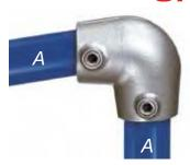
Used to join the top rail to an end upright on a guardrail on a slope from 0° to 11°. Pipe cannot be joined within this fitting.
