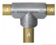
Commonly used as the 90° joint between the top rail and an intermediate upright on safety railing. As there are two socket set screws in the sleeve, this fitting can be used where a join is required in the horizontal pipe. The type L10 fitting can be used as an alternative when a join in the pipe is not required.
