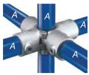
The unique hinge and pin system of this fitting enables existing structures to be easily extended without the need for dismantling. This fitting is most frequently used in multiple upright structures to tie a center upright with horizontal pipes in four directions. The upright passes through the fitting.
