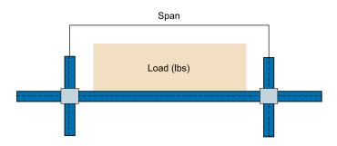
The values in Table 17 are an indication of a UDL that a rack consisting of two support pipes can support.
