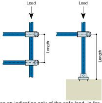
Table 19 gives an indication only of the safe load, in lbs., that may be carried between the above restraints by single Schedule 40 pipes when used as uprights.
