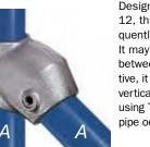
Designed as an alternative to Type 12, this adjustable fitting is most frequently used for bracing and struts. It may be used at any selected angle between 30° and 60°. As an alternative, it is possible to use Type 29 in its vertical position in place of Type 27, using Type 27 only where a join in the pipe occurs.
