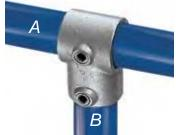
Designed to give a 90° butt joint between two pipes. Frequently used for the joint between end uprights and the middle rail where the railing site is straight and level. Also used for base ties on racking. This fitting cannot be used where through pipe is required to be joined within the fitting. Type 25 should be used when a join in the pipe is necessary.
