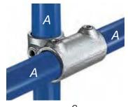
Designed to give a 90° offset crossover. As there are two socket set screws in the sleeve, this KEE KLAMP fitting can be used where a join is required in the horizontal pipe. For economy, it is possible to use a Type 45 in place of the 145, using the 145 only where a join in the pipe occurs. When calculating the cutting lengths for pipe, dimension 'G' should be added to give the pipe length for the upright.
