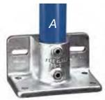
Designed for guardrail and balustrade applications with the added benefit of attaching a toe board to the base. The base plate holes are sufficient diameter to allow for attachment with either a mechanical or chemical anchor. The side plates have slotted holes to allow for a degree of sideways movement for ease of installation. (See page 36 for Toe Board).
