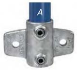
Type 115 is designed for palm fixing of guard rail and balustrades to walls, parapets, steps, and ramps. The upright cannot drop through the socket. Packer plates, Type S115, are available to allow the fitting to be positioned in channels, slots, and other offset areas.
