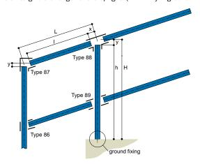
Table 4 gives details of dimensions required for calculating the rail lengths, where angles are between  $0^{\circ}$  and  $11^{\circ}$ .
