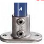
Ideal when a structural fixing is required for guard rail and balustrades. The holes are of sufficient diameter to insure proper fixing with either mechanical or chemical anchor. The two set screws in the vertical socket give greater side-load stability to the upright. It is recommended that the fixing holes in the flange should be in line with the applied load (refer to table on page 43).
