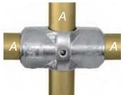
Usually paired with type L25 to give a 90° joint between the middle rail and an intermediate upright on safety railing. The upright passes through the fitting.
