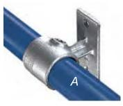
Designed to carry handrails along walls or to fix structures back to walls. The pipe passes through the fitting and cannot be joined with the fitting. Type 70 is also used to attach toe boards to the base of guardrail uprights. Holes provided for countersunk flat head screw fixings only.
