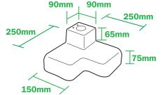
PVC BASE - 250-6 Recycled PVC base provides the support for the Vertical Standards.
