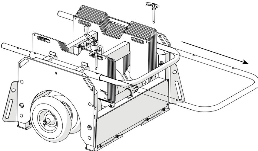
Pull the U shaped handle outward stopping when the last set of mounting holes is visual through the outer handle tube.
