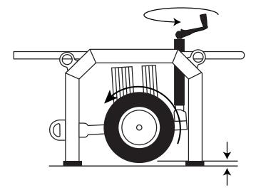
To relocate the BIGFOOT flip the handle so that the knob faces up. Rotate the handle clockwise until all four wheels are lowered to the surface and the frame of the Bigfoot is raised from the surface. Lowering the wheels raises the ballast weights.
