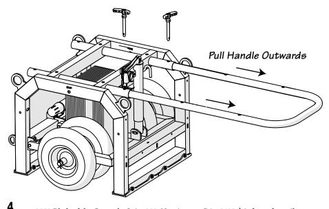
Pull the U shaped handle outward stopping when the last set of mounting holes is visual through the outer handle tube.
