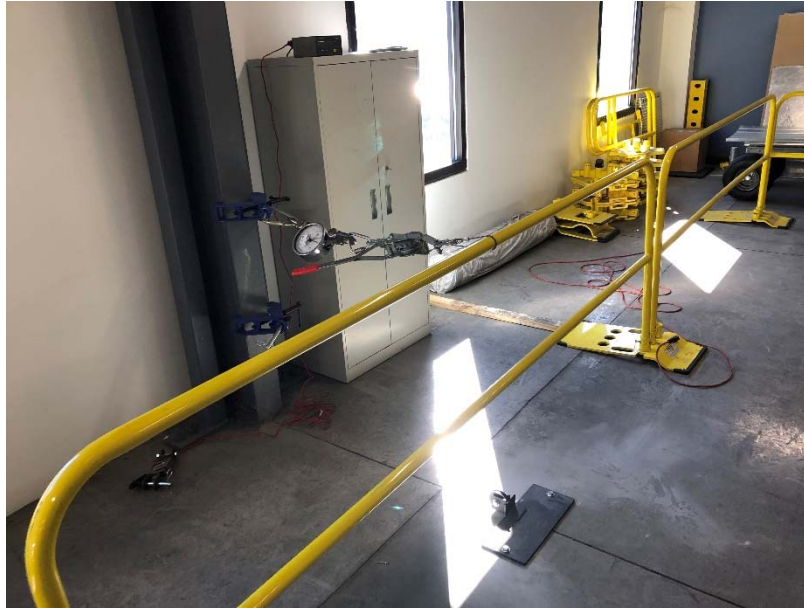
PHOTO 1: Horizontal 200lbs. Test on Upper Rail Section.
