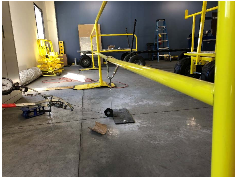
PHOTO 4: Vertical 150lbs. Test on Lower Rail Section.
