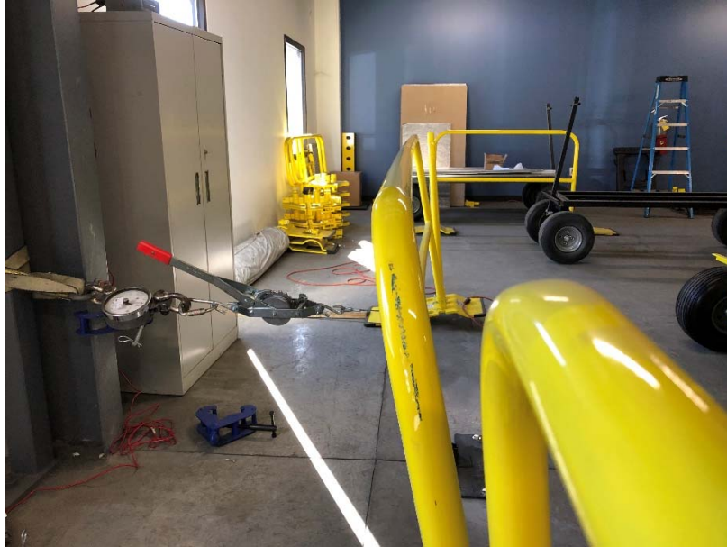
PHOTO 3: Horizontal 150lbs. Test on Lower Rail Section.
