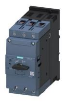
Circuit breaker size S3 for motor protection, CLASS 10 A-release 75...93 A N-release 1300 A screw terminal Standard switching capacity
