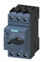
Circuit breaker size S0 for motor protection, CLASS 10 A-release 0.45...0.63 A N-release 8.2 A screw terminal Standard switching capacity
