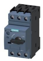
Circuit breaker size S0 for motor protection, Class 10 A-release 0.14...0.2 A Short-circuit release 2.6 A Screw terminal Standard switching capacity
