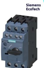
Circuit breaker size S00 for motor protection, CLASS 10 A-release 7...10 A N release 130 A screw terminal Standard switching capacity with transverse auxiliary switches 1 NO+1 NC  $\,$
