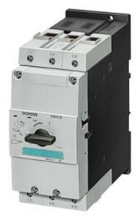
Circuit breaker size S3 for motor protection, Class 10 A-release 45...63 A Short-circuit release 819 A Screw terminal Standard switching capacity !!! Phased-out product !!! Successor is SIRIUS 3RV2 Preferred successor type is >>3RV2031-4JA10<<
