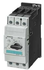
Circuit breaker size S2 for motor protection, Class 10 A-release 36...45 A Short-circuit release 585 A Screw terminal Standard switching capacity !!! Phased-out product !!! Successor is SIRIUS 3RV2 Preferred successor type is >>3RV2031-4VA10<<
