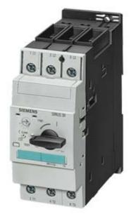
Circuit breaker size S2 for motor protection, Class 10 A-release 28...40 A Short-circuit release 520 A Screw terminal Standard switching capacity !!! Phased-out product !!! Successor is SIRIUS 3RV2 Preferred successor type is >>3RV2031-4UA10<<
