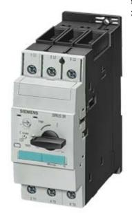
Circuit breaker size S2 for motor protection, Class 10 A-release 18...25 A Short-circuit release 325 A Screw terminal Standard switching capacity !!! Phased-out product !!! Successor is SIRIUS 3RV2 Preferred successor type is >>3RV2031-4DA10<<
