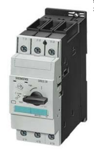
Circuit breaker size S2 for motor protection, Class 10 A-release 14...20 A Short-circuit release 260 A Screw terminal Standard switching capacity !!! Phased-out product !!! Successor is SIRIUS 3RV2 Preferred successor type is >>3RV2031-4BA10<<
