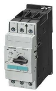
Circuit breaker size S2 for motor protection, Class 10 A-release 11...16 A Short-circuit release 208 A Screw terminal Standard switching capacity !!! Phased-out product !!! Successor is SIRIUS 3RV2 Preferred successor type is >>3RV2031-4TA10<<
