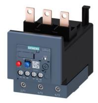
Overload relay 45...63 A Thermal For motor protection Size S3, Class 10 Contactor mounting Main circuit: Screw Auxiliary circuit: Screw Manual-Automatic-Reset
