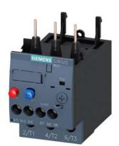
Overload relay 7.0...10 A Thermal For motor protection Size S0, Class 10 Contactor mounting Main circuit: Screw Auxiliary circuit: Screw Manual-Automatic-Reset
