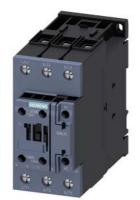
power contactor, AC-3 50 A, 22 kW / 400 V 1 NO + 1 NC, 24 V AC, 50 / 60 Hz, 3-pole, Size S2, screw terminal
