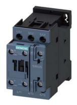
power contactor, AC-3 25 A, 11 kW / 400 V 1 NO + 1 NC, 220 V AC, 50 Hz 240 V, 60 Hz 3-pole, frame size S0 screw terminal
