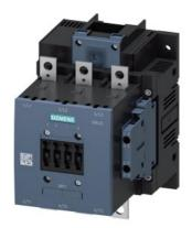
power contactor AC-1 275 A / 690 V / 40  $^{\circ}$ C 3-pole, Uc: 110-127 V AC(50-60 Hz) / DC drive: conventional auxiliary contacts 2 NO + 2 NC main circuit: busbar control and auxiliary circuit: screw terminal
