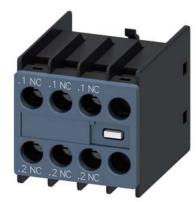
Auxiliary switch on the front, 3 NC Current path 1 NC, 1 NC, 1 NC for 3RH and 3RT screw terminal .1/.2, .1/.2, .1/.2
