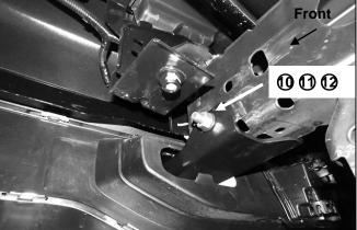
(Fig 7) Inner passenger/right side Bracket with Single Bolt Plate pictured from behind camper
