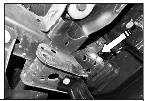
(Fig 3) Passenger/right outer mounting bolts for tow hook pictured from behind bumper
