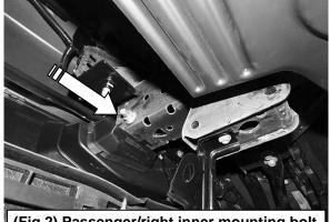
(Fig 2) Passenger/right inner mounting bolt for tow hook pictured from behind bumper
