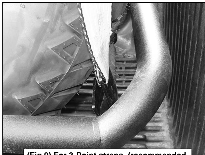
(Fig 9) For 3-Point straps, (recommended separate purchase). Attach the hooks to either the upper hoops or inner plates as shown in picture above
