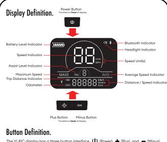
The YL81C display has a three button interface. 1 (Power), + (Plus), and - (Minus). It will light up for night visibility when buttons are pressed.
