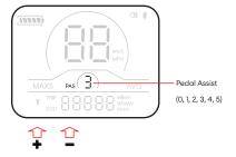
NOTE: By default, the system will reset PAS to level 1 every time it is powered on.
