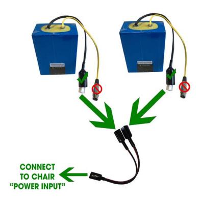
Two 10 Ah Batteries are shown in the illustration above.
