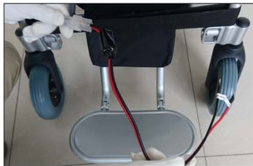
12. If you will use your own battery pack, you need the battery cable we provided to match the battery connector (c).
