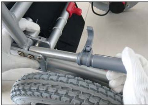
9. Install the extendable standing legs and fix them with the knobs.
