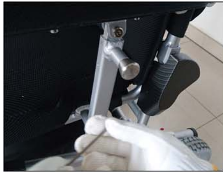
7. Install the plastic covers with included screws.
