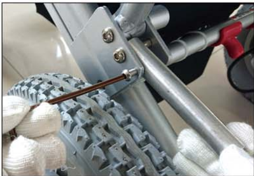
8. Install the metal standing legs with included screws.
