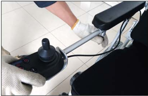
6. Insert the controller joystick into the armrest tube.
