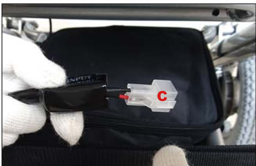
11. Plug the battery connector (c) to the battery pack we sent in separate package.
