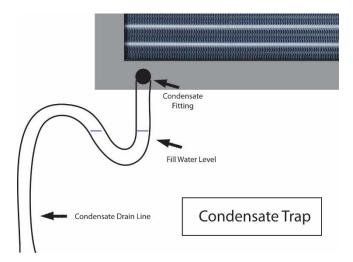
As shown above, the drain line should drop, then rise (but stay below the height of the fitting), and then drop again, and must terminate in air, not liquid After installing the trap, it must be charged with water as shown.
