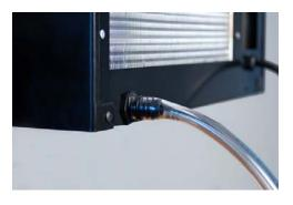
Our REAR drain line comes with the fitting installed in the rear of the cooling unit. Our BOTTOM drain line requires installation of the fitting. To install, apply pipe joint sealant (included) to the male threads of the barbed fitting, then hand-tighten the fitting into the threaded drain line hole. Do not force – if cross threaded, back out and realign. Finish by tightening the fitting with a wrench.
