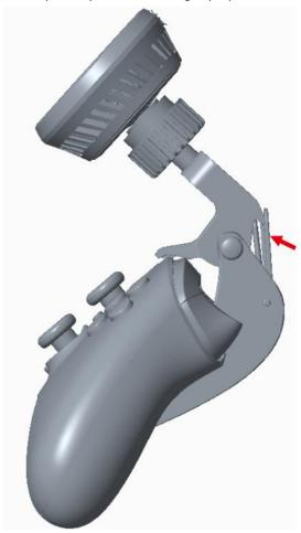
$5_{\times}$  Step five, push the locking clip up again to secure the bracket and handle.
