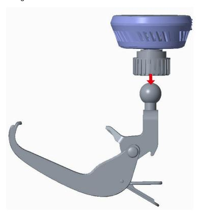
2. Step two, install the handle onto the bracket.
