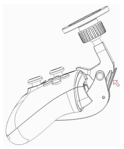
5. Step five, attach the magnetic sheet from the packaging box to the back of the phone, then let the phone adsorb onto the bracket.
