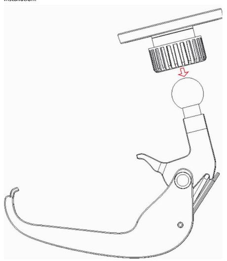
2. Step two, install the handle onto the bracket.
