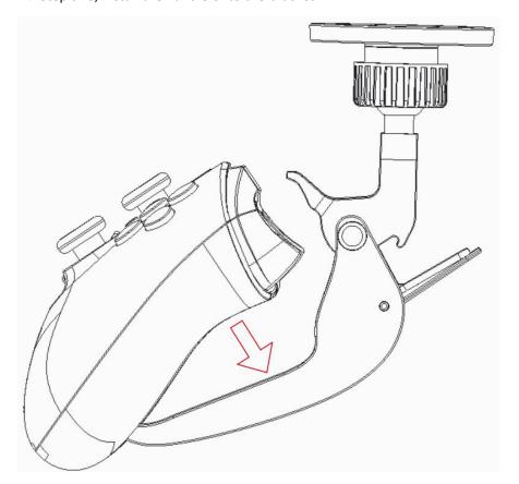
3、Step three, push the metal ring into the groove.
