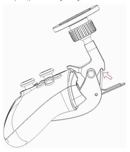
4. Step four, push the locking clip up to lock the bracket and handle.
