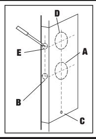
Converting from an existing standard door knob to a handleset.
