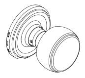
a. Push the Removal Tool against the Knob Catch to depress it. Pull the knob off the Spindle.
