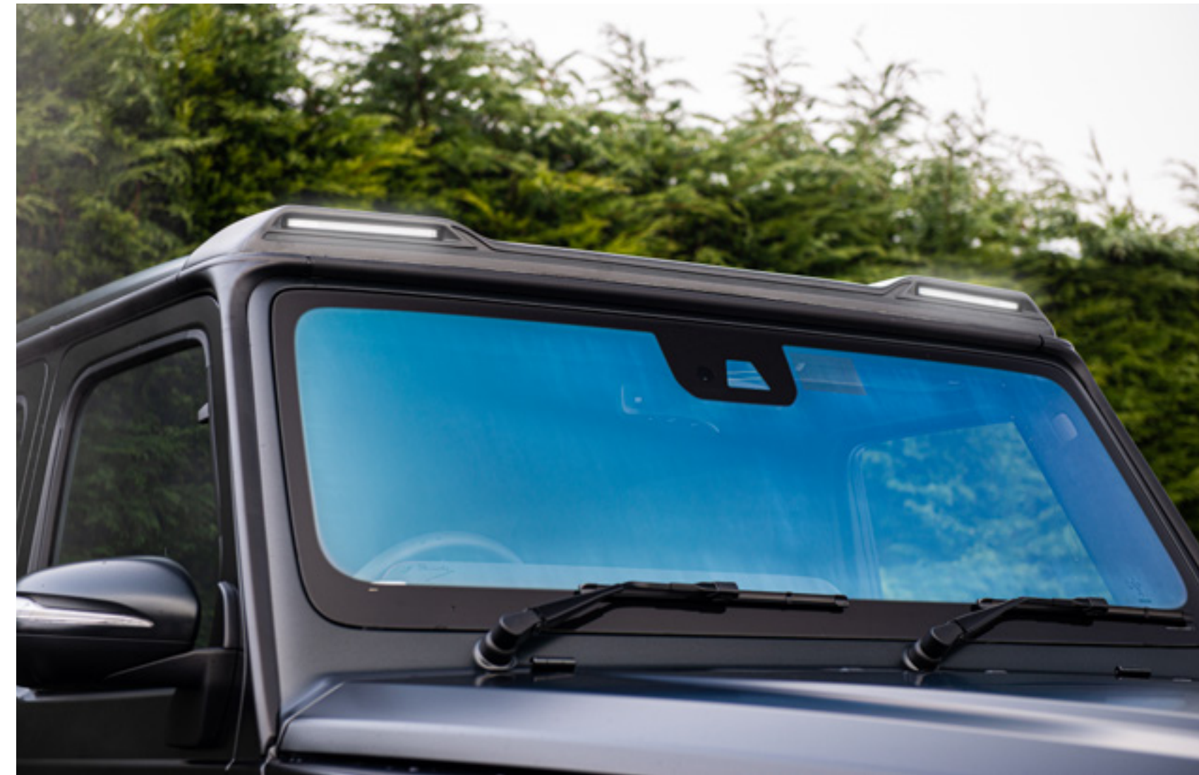
FRONT ROOF SHIELD WITH LED LIGHTS MATERIAL: ABS COMPOSITE PART NUMBER: BCRMG2PF
