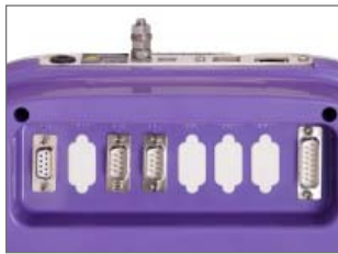
4 D-SUB connectors - IP40
