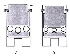
The surfaces that the balls run on should be smooth and flat. Deep grooves indicate bad wear, likewise miniature or chipped balls. Good innards raise the top part level with, or even slightly *proud* of, the outside body ... but if you find it is sunk *inside* ... then it needs replacing. Pack well with grease.
