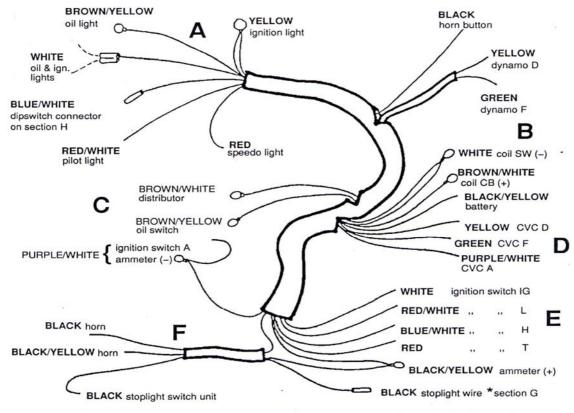
(To complete the wiring of the stoplight switch run the short piece of black wire from the other side of the stoplight switch to the black/yellow side of the horn)
