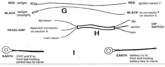
Wiring harness for all models 1949 to 1957 incorporating a stoplight switch, 6 V or 12 V
