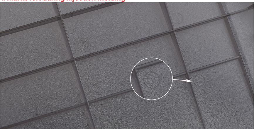
2. There will be the sprue marks inside the case after the injection, but once the keyboard is assembled, the marks are not visible
