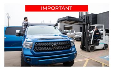
Roof top tents can be very heavy and awkward. Installing one on the roof of your truck can be very dangerous and you can hurt yourself and your truck. Do not do this alone or without help from others or proper tools to get the tent elevated and on your roof rack.
