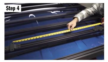
Measure the width of the rails on your tent, you want to measure from the center of the bolt on one rail, to the center of the bolt on the opposite rail. Then you will do the same with your mounts on the roof rack. You will want to center the mounts on your roof rack, and also make sure they are the same width as the rail. Then tighten the bolts. It is very difficult to tighten the bolts after the tent is installed.
