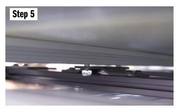
Lift the rack up into position. Then slide the 8ea t-nuts.bolts into position and through the holes in the mounts. Then install the lock nuts. Finally tighten the 8ea bolts on the tent to the mounts.
