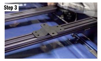
Now we will set up the mounts on your roof rack. Position the mounts as far apart as possible, and over the roof rack feet as much as possible. This will help your rack distribute the load more efficiently and make your tent a little more stable while in use. Once you have your positions, slide in the drop-in t-nuts, then install a bolt and washer for all 4ea positions on the mount. Do this for all 4ea mounts. Leave the hardware loose enough to adjust your mounts.
