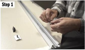
First we need to prep the tent. You will need to follow all of your tents installation instructions. When it is time to install the t-nuts into your tent rails, we recommend using the included 5/16" bolts as they are shorter and will not hit your roof. Slide the bolt in, ensuring it fits inside the nut, then slide the nut into the rail.
