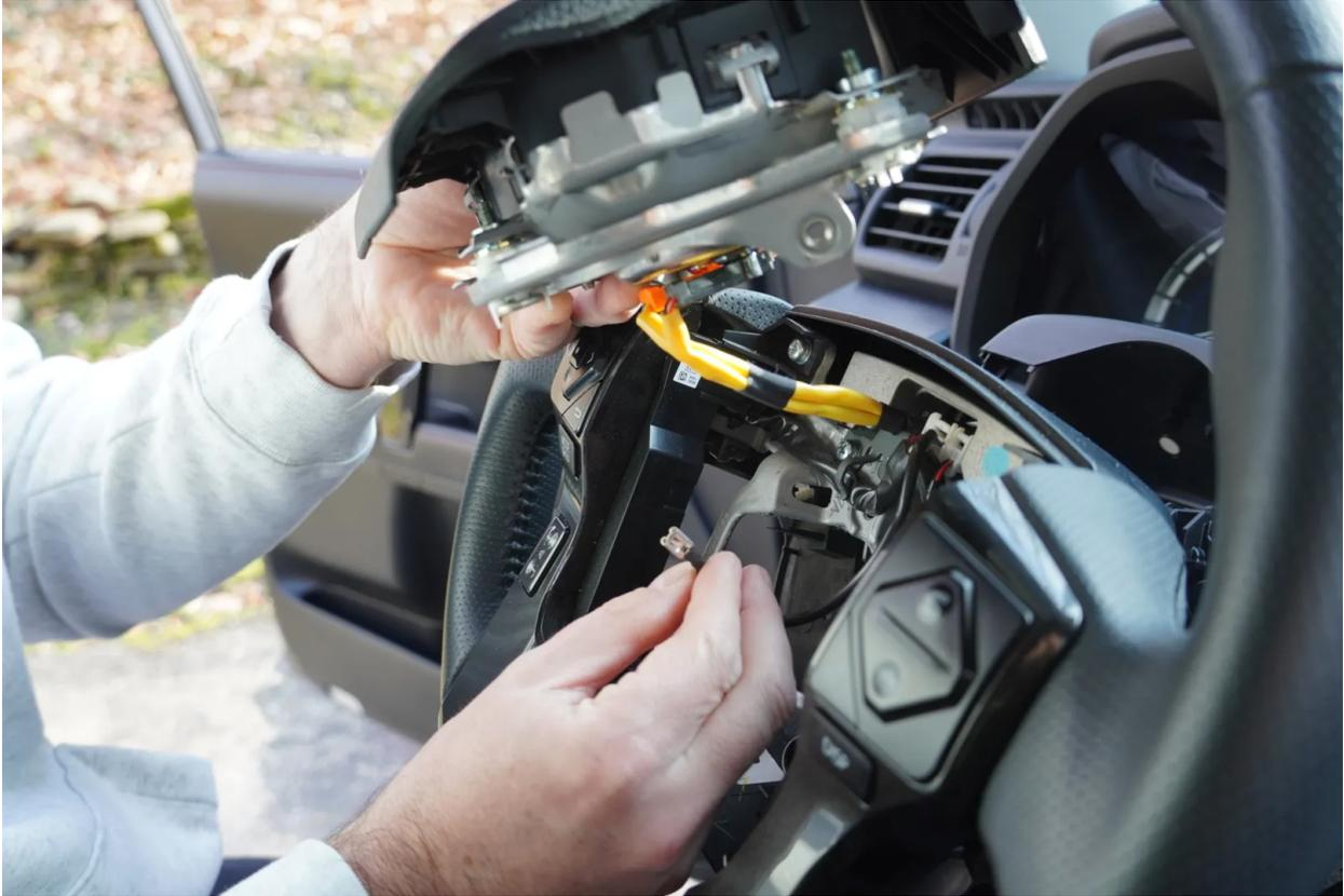
Now that the two (2) T27 Torx screws have been backed out, the airbag can be removed.
