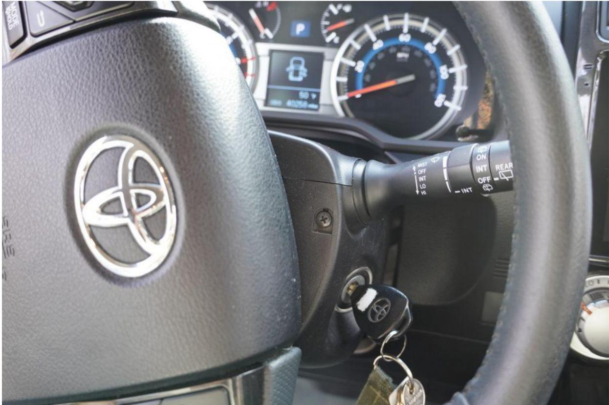
Next, turn the steering wheel to the right exposing the right-side screw, and remove it. Both screws will be reused, so put them aside for later use.
