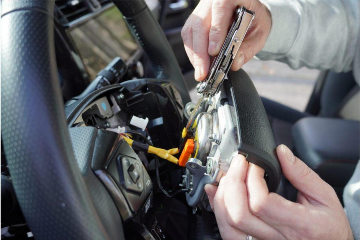
Using a flathead screwdriver, wedge in between the yellow clip holding the airbag wires (black and orange) onto the airbag. Eventually, the clip will pop back and you can remove the wire. Perform the same step on the remaining wire.
