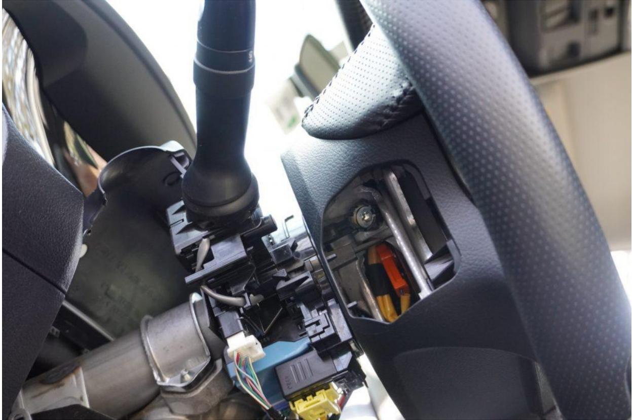
Remove the two (2) T27 Torx screws. Both screws can be loosened but not removed completely since they are held in place with clips (likely so as not to drop inside the steering wheel column housing).
