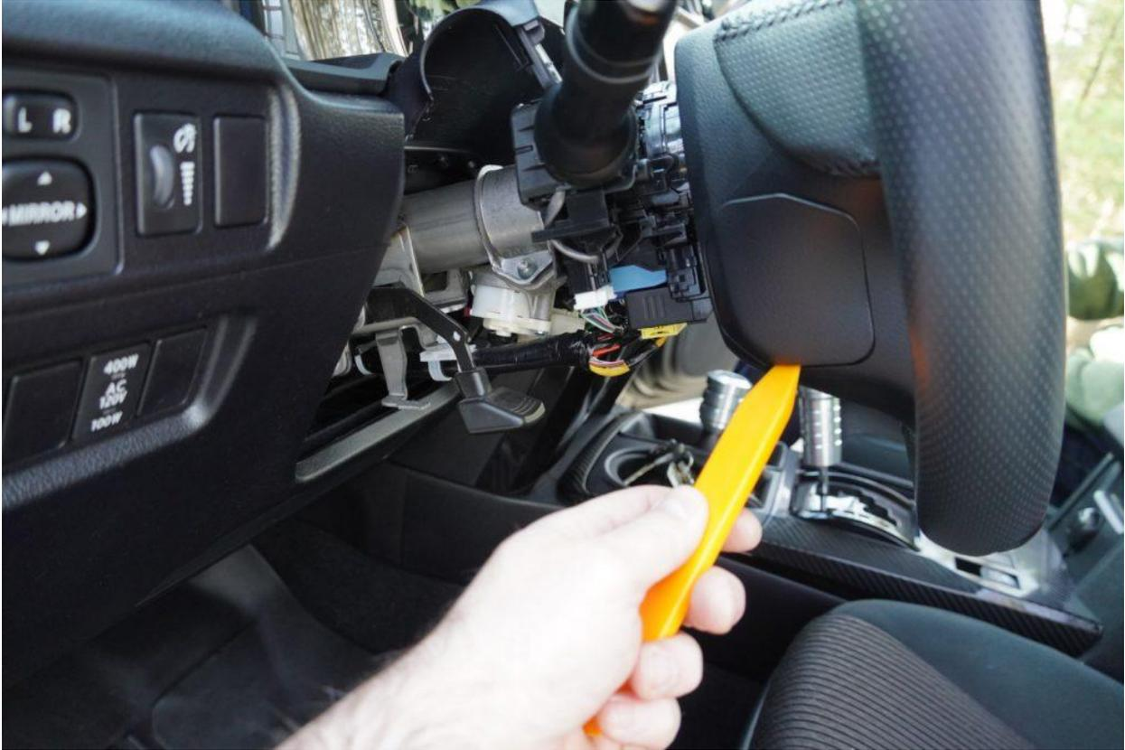
Using the plastic panel removal tool, remove the left and right side panels affixed to the steering wheel.
