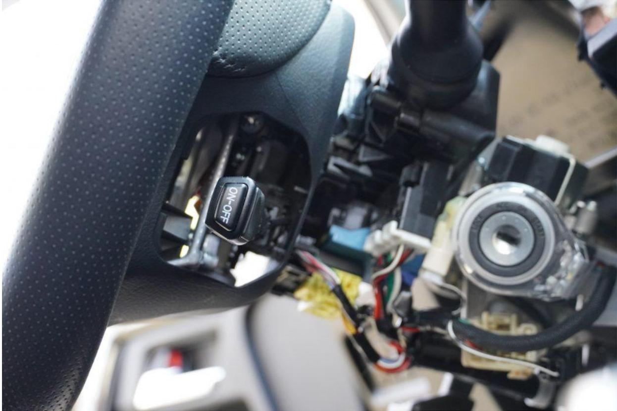
This will expose a T27 Torx screw on each side that needs to be removed.
