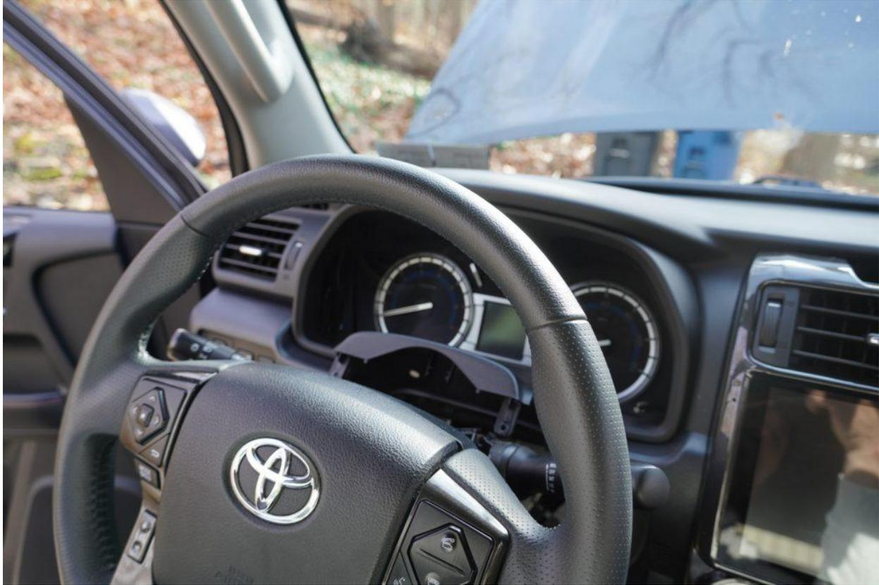
Next, loosen the upper panel. This panel is tied into a pleather dust protector which doesn't need to be disconnected altogether to finish the proceeding steps. So, simply lift it up and push it back towards the gauge cluster so it's out of the way.
