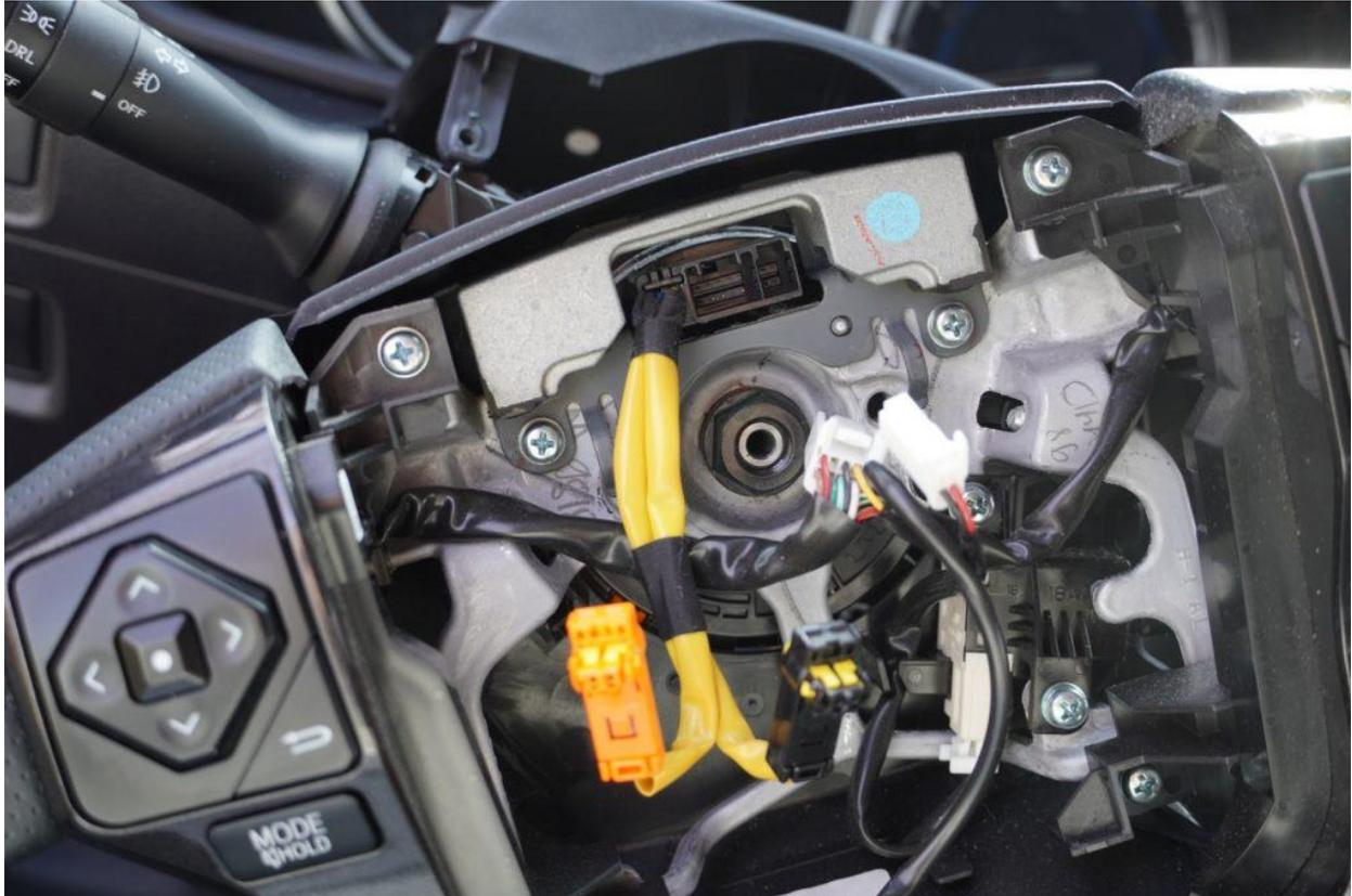
With the airbag removed, disconnect the two (2) steering wheel control clips. One of the clips is used for the cruise control functionality and the other supports all of the steering wheel convenience controls.
