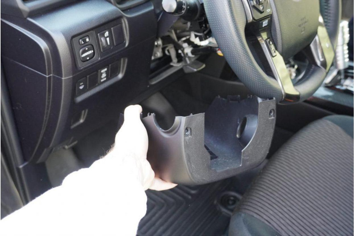
With both of the steering wheel panel screws removed, both the upper and lower panel can be removed.
