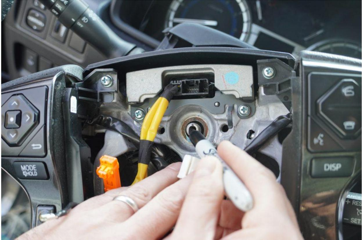
With the wheel nut removed, mark the center on the steering wheel with a permanent marker to ensure it aligns with the new wheel you'll be installing.
