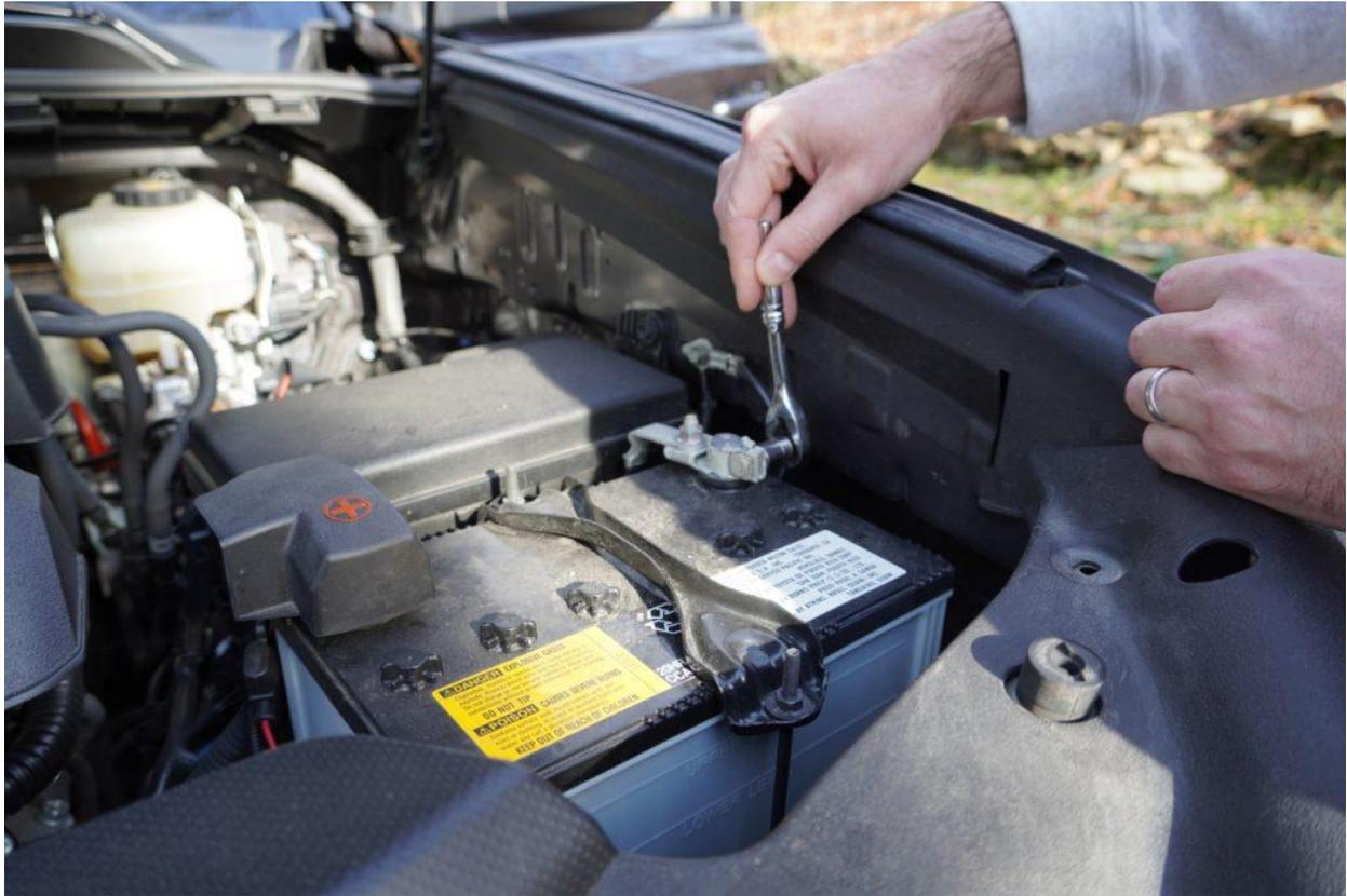
Now that the engine is off, disconnect the battery. Why? You're going to be removing the steering wheel, the main airbag is hiding right behind the steering wheel, and you don't want that thing blowing up mid-install.
