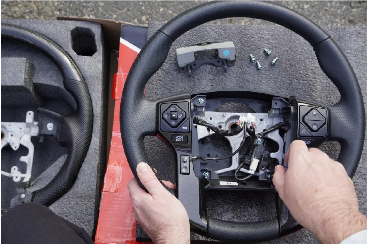
Now it's time to swap over all of the components from the OEM wheel to the new carbon fiber wheel.
