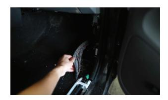
**5.** Remove plug covering body mount bolt.
