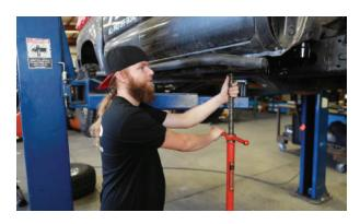
**22.** If desired the excess body mount bolt can be cut off.
