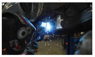
**20.** The inside and outside of the front and rear of the bracket along with the inside of the top will need to get welded.
