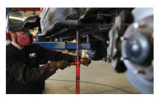
**13.** The body mount can be cut off using a plasma cutter, cutting torch, sawzall, or angle grinder. If using a sawzall or angle grinder the body mount bracket may need to be cut off in sections. Ensure that no wiring or any other important items will be damaged by the cutting process.
