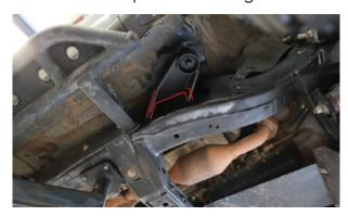
**21.** Once welding is complete the jack supporting the body can be removed.
