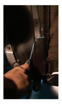
**8.** Mark and cut fender as shown. Cut off wheel on a grinder works well for this. Not all applications will look exactly the same as this picture. Different models may require slightly different fender trimming, but we recommend trying to trim the fender on the same plane that the body mount will be cut. This cut may also need to be adjusted for larger tires. (Vehicle used in instructions is 2017 Tacoma.)
