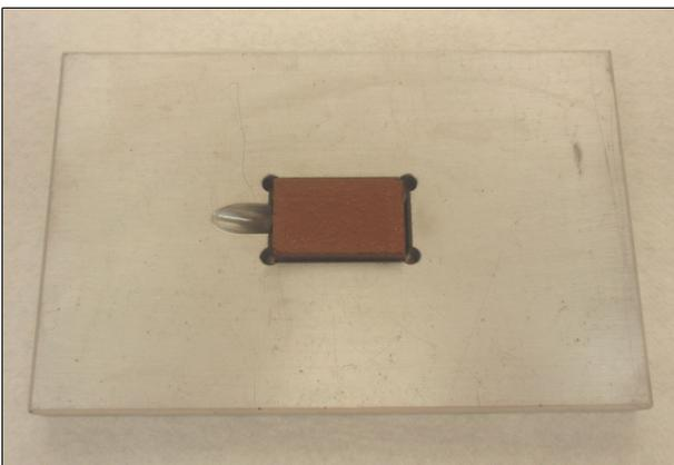
Photo 3. Mounted carrier in stainless steel holder.
