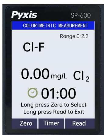
Figure 14. CHLORINE MEASUREMENT screen
