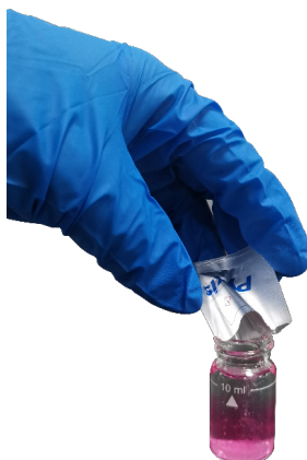
Figure 17. Add DPD powder to sample
