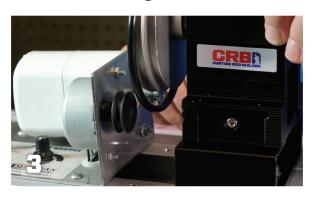
3. Before locking the new chuck down, put the old belt from the American Tackle/Pac Bay wrapper into place and line it up. Note: Pay attention to the pully as to not accidentally place over the plate mounting screws.
