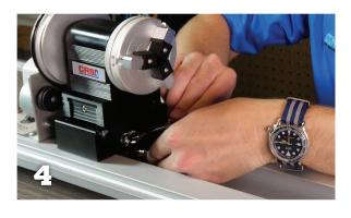
4. Once the belt is aligned, use a 10mm wrench to tighten the front and back bolts at the base of the chuck.
