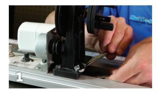
To get started, remove the rod stands and separate the tracks on the American Tackle or Pac Bay wrapper. Use a 10mm wrench to remove the bolts holding on the chuck.
