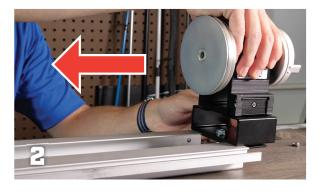
Once you remove the old chuck, you can slide your new CRB Chuck Upgrade down the track and into place where the old chuck was located.
