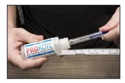
**PRO TIP:** Withdraw and inject epoxy slowly with syringes to avoid adding air bubbles.
