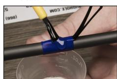
**PRO TIP:** Do not glob on epoxy, apply evenly to thread and touch up bare thread spots as you go.
