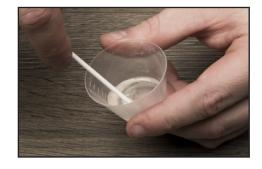
**PRO TIP:** Keep your excess epoxy handy to check its hardness and avoid tampering with the actual finish on the thread wraps.
