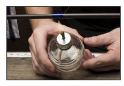
**PRO TIP:** Never apply heat directly to the epoxy, as too much will create more bubbles or harm components.
