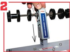
At this point you will slide the stacker over the existing center post on the HWS-1 Hand wrapper. The tolerances are very tight between the two of these parts and may require some manipulation of the product.\*
