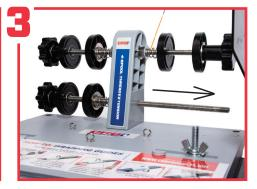
Once you have slid the TC4 unit over the center post look to make sure the holes in each unit align, then slide the threaded rod through and lock into place with the included locking nut on either side of the post.
