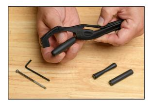
2. To change a roller head, use the provided allen key to remove the screw. This screw will completely come out of the tool with the roller head and washer. You can now slide the roller head off the screw and reinstall with a different roller head.
