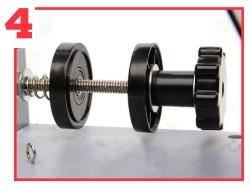
Install the remaining components to the bottom post in this order: Steel Washer, Conical spring, Washer, thread cap (smooth surface facing toward the end of the rod), thread cap (smooth surface facing toward the first thread cap), Large washer, spacer, washer, locking knob.
