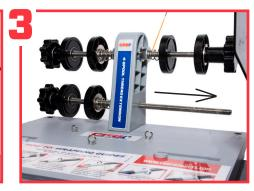
Once you have slid the thread adapter over the center post look to make sure the holes in each unit align, then slide the threaded rod through and lock into place with the included locking nut on either side of the post. Then Install the tension rod into the pre-drilled hole with the provided adhesive.
