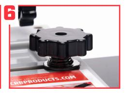
Now mount two of the Rod Stands to the HWS Base. Align the rear hole on the rod stand with the bottom slot on the AHWS Base and slide a Rod Stand Bolt through both pieces. Secure by installing a steel washer, conical spring, washer, and locking knob in that order starting from the base.
