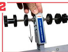
At this point you will slide the stacker over the existing center post on the AHWS Hand wrapper. The tolerances are very tight between the two of these parts and may require some manipulation of the product.\*
