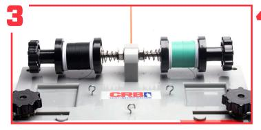
Once you're ready to wrap, just add up to four spools of thread between the two Ball Bearing centered Thread Caps and begin wrapping. The AHWS is designed to retain all functionality that is originally found on a stock HWS-1.
