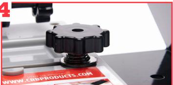
Now mount two of the Rod Stands to the AHWS Base. Align the rear hole on the rod stand with the bottom slot on the AHWS Base and slide a Rod Stand Bolt through both pieces. Secure by installing a steel washer, conical spring, washer, and locking knob in that order starting from the base.
