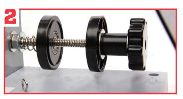
Install the remaining components to the bottom post in this order: Steel Washer, Conical spring, Washer, thread cap (smooth surface facing toward the end of the rod), thread cap (smooth surface facing toward the first thread cap), Large washer, spacer, washer, locking knob.
