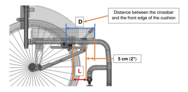
3. Position part #2 on top of part #3 at the distance **L** from the edge. Take the screws and locknuts from the bag attached to part #2. Insert the screws from below into the holes closest to marked location. Tighten the screws with an Allen key as you hold the locknuts in place with the open-end wrench.
