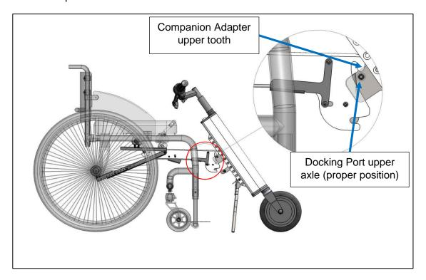
6. Insert the screws through the holes in the Power Module that align with the holes of the Docking Port plates. Secure with the locknuts but do not tighten them yet.
