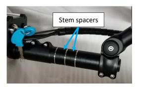
5. You also may adjust the height of the handlebar by adding or removing stem spacers from the stem extender. (see right picture above).
