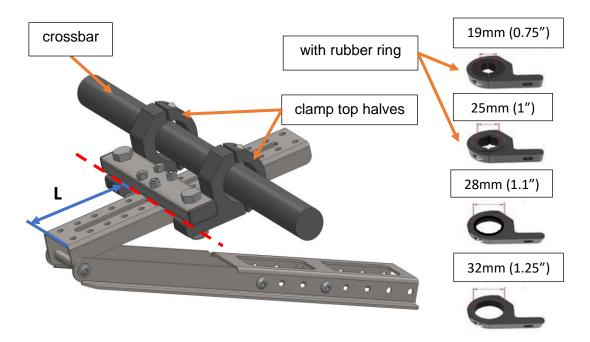
5. Align part #1 and part #4 together. Slide them one into another until part #3 is parallel to the ground. Once this position is achieved, locate two matching pairs of holes in part #4 and part #1. Fasten using the screws and locknuts from the bag attached to part #4. Tighten the screws with an Allen key while holding the locknuts in place with the openend wrench.
