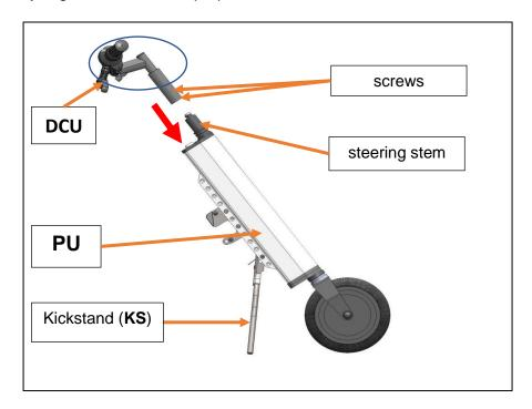
3. Tighten the clamp screws on the stem.
