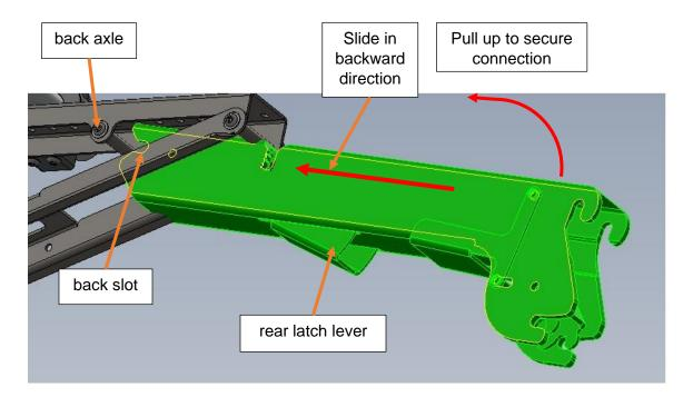
2 **To detach** the Companion Adapter from the Docking Module, press the rear latch lever, then push the Companion Adapter down and pull it out.
