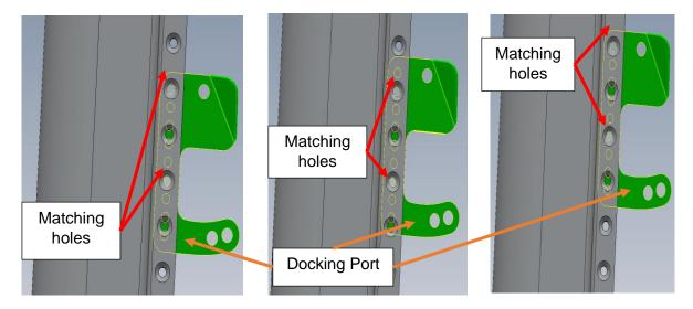
4. Once you have achieved optimal position of the Docking Port, tighten the screws with an Allen key while holding the locknuts in place with the open-end wrench.
