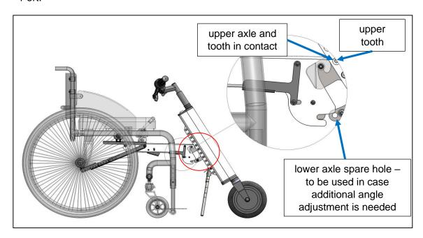
2. Use both hands to push the handlebar forward and slightly up from the wheelchair as shown (the Companion will pivot on the upper axle.) until you hear a click; this will mean that the locking mechanism is activated and the Adapter and the Power Unit are connected. The casters of your wheelchair should lift off the ground. The recommended gap between the casters and the ground is about **five centimeters** (two inches).
