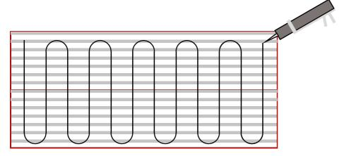
Now gently press the panel in place against the wall. Starting from the ground if mounted on top of each other in horizontal direction. Hold the panel for 3min to let the high tack adhesive form it's initial bond and then all should be firmly secured. Let rest for at least 1 day before bonding is complete.
