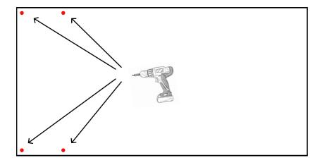
Once completed, reposition the acoustic panel against the wall and screw it in place with the four screws. Check if everything is correct and proceed with drilling the holes and marking the wall for the remainder of screws.
