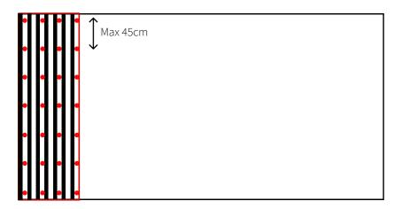
We recommend placing 4 screws horizontally per panel. Maximum 45 cm between horizontal lines of placement. Repeat for every acoustical panel until the end of the wall.
