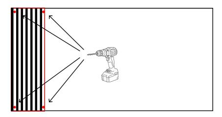
Now remove the panel and drill the holes in the wall with the correct type of plug if necessary.
